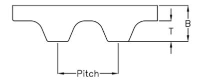
Height B mm= 2.2Height T mm= 1.2Length= 560Number of teeth= 112Pitch= 5Type= PU 20 T5 560Width= 20
